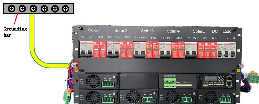
Figure 1-2 Installing a protective ground cable
