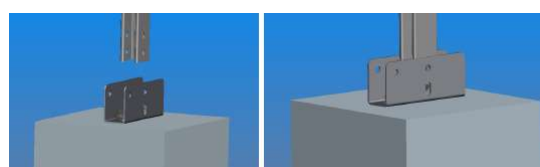
Front & Rear leg fixings into foundations
